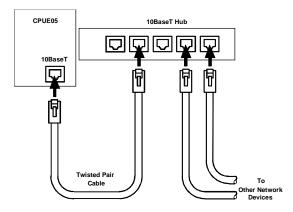
The cable between each node and a hub or repeater can be up to 100 meters in length. Typical hubs or repeaters support 4 to 12 nodes connected in a star wiring topology.
